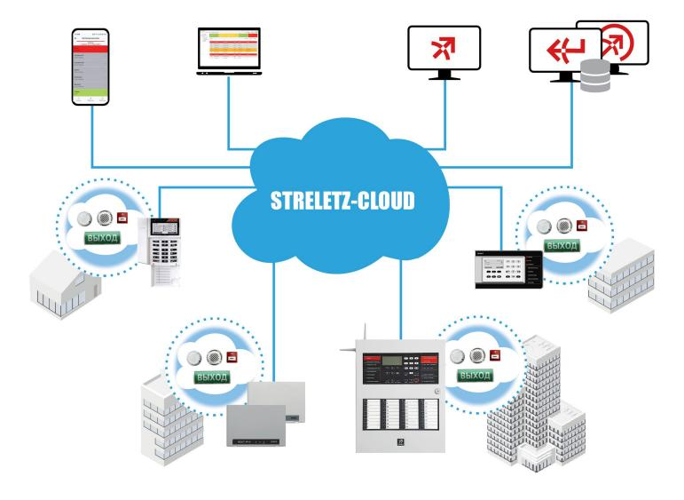
Cloud technologies for remote control and monitoring via a mobile phone, a computer or a web-browser
